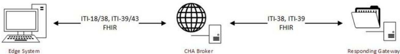
CommonWell member organizations that want to respond to document query & retrieval requests MUST register their respective XCA/FHIR Responding Gateway services. In addition to supporting the required query and retrieve XCA transactions (ITI-38 and ITI-39) or FHIR transactions
